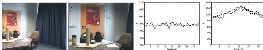
**Fig. 3.** Left: Images from the zoom-pan sequence for rotation calibration, right: calibration results for constant and varying focal length
