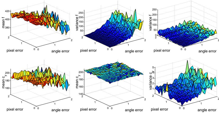
**Fig. 1.** Noise robustness measurements. Top from left to right: mean of linear estimated focal length  $f$ , variance of linear estimated focal length  $f$ , variance of MAP estimated focal length  $f$ . Bottom from left to right: mean of linear estimated principal point component  $c_y$ , mean of MAP estimated  $c_y$ , variance of MAP estimation
